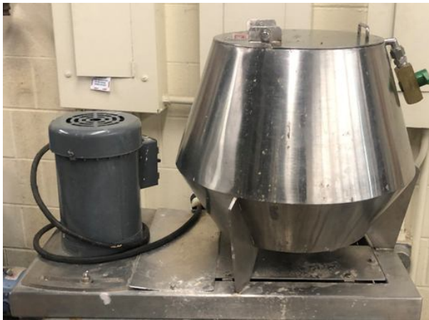
Fig. 4. Low Consistency Laboratory Repulper [35]
