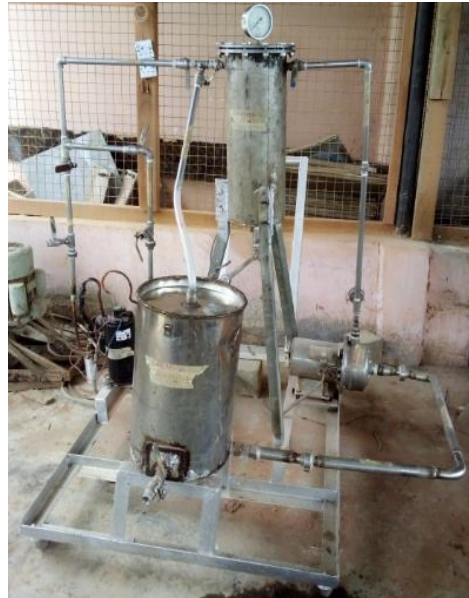
Diagram Plate 1. Chemical Impregnating Equipment used.
