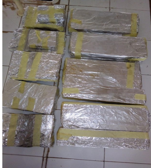
Diagram Plate 2. Treated wood wrapped with aluminium.
