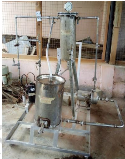
Plate-Figure 1 . Chemical Impregnating Equipment used. Source: Own autorship.
