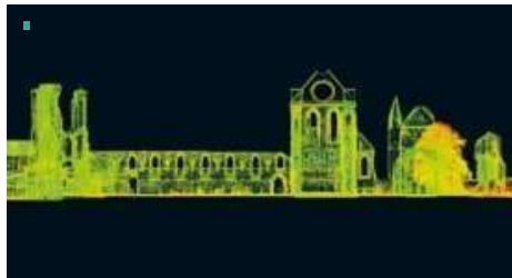
■ Fig. 7. An orthographic point cloud image displayed with intensity values and silhouette shading
