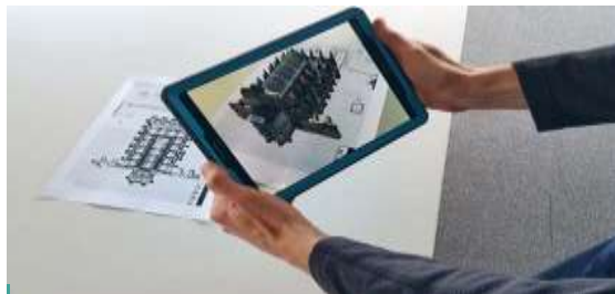
Fig. 25. Augmented reality application overlaying a 3D model of Rosslyn Chapel on top of a tracked 2D target. Picture by courtesy of Historic Environment Scotland [1]
