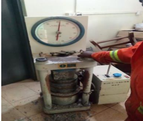
Fig. 6 – Compressive strength test Fig. 7- Measuring the weight of the test specimen
