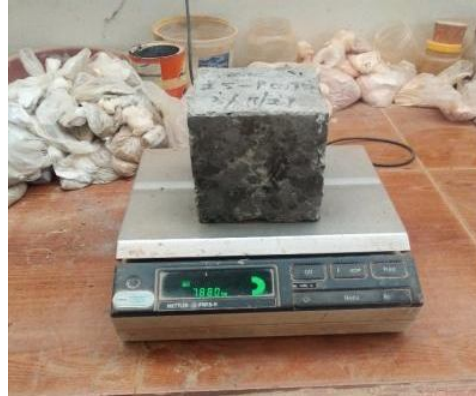
Fig. 6 – Compressive strength test Fig. 7- Measuring the weight of the test specimen
