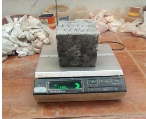
Fig. 7- Measuring the weight of the test specimen
