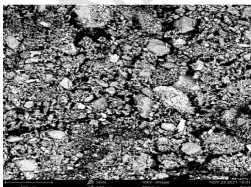
Fig. 3. SEM analysis of raw Achalla clay (ACC) (@100 μm)
