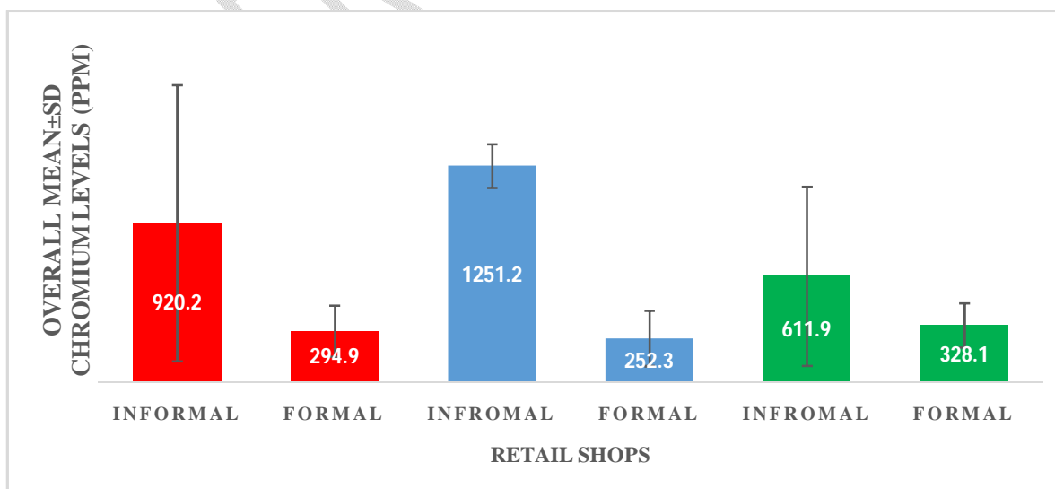
Fig. 1: Overall chromium mean \pm SD levels (ppm) in various automotive paint colours purchased from informal and formal retail shops
