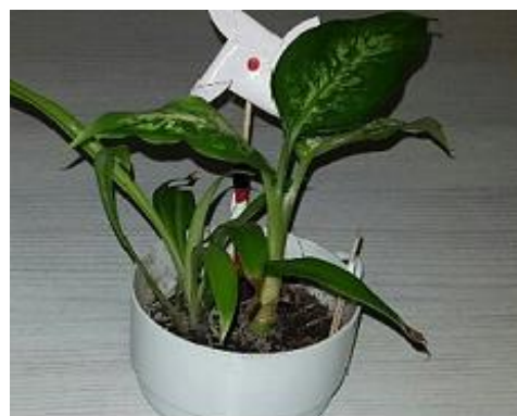
Figure 3. PPB with double pair of electrodes in the soil (not visible) and a small coil at the end of the line behind the stem.
