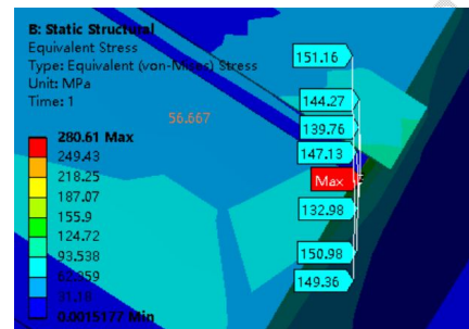
Figure 18 Local enlargement of concentrated stress
