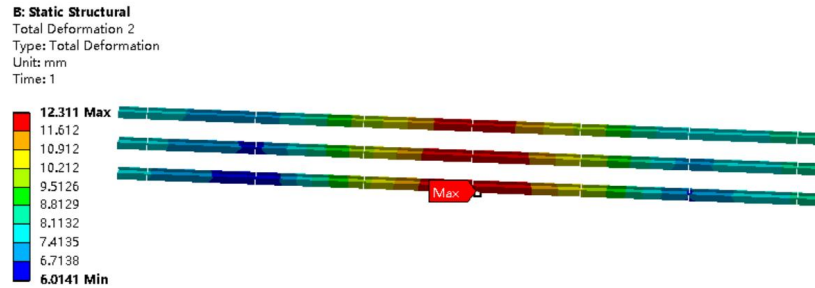
Figure 12 Secondary beam structural displacement cloud
