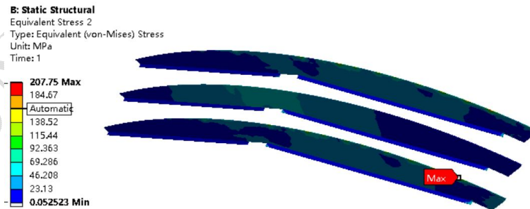
Figure 13 Main beam stress cloud
