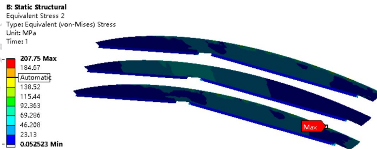
Figure 13 Main beam stress cloud
