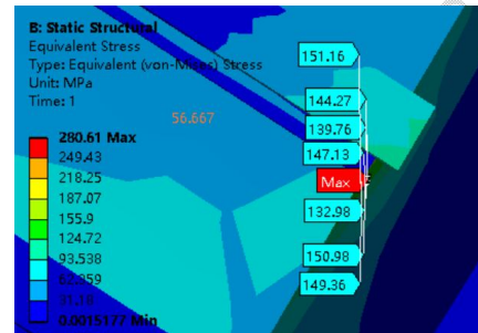
Figure 18 Local enlargement of concentrated stress
