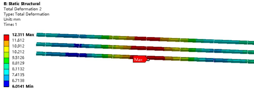
Figure 12 Secondary beam structural displacement cloud
