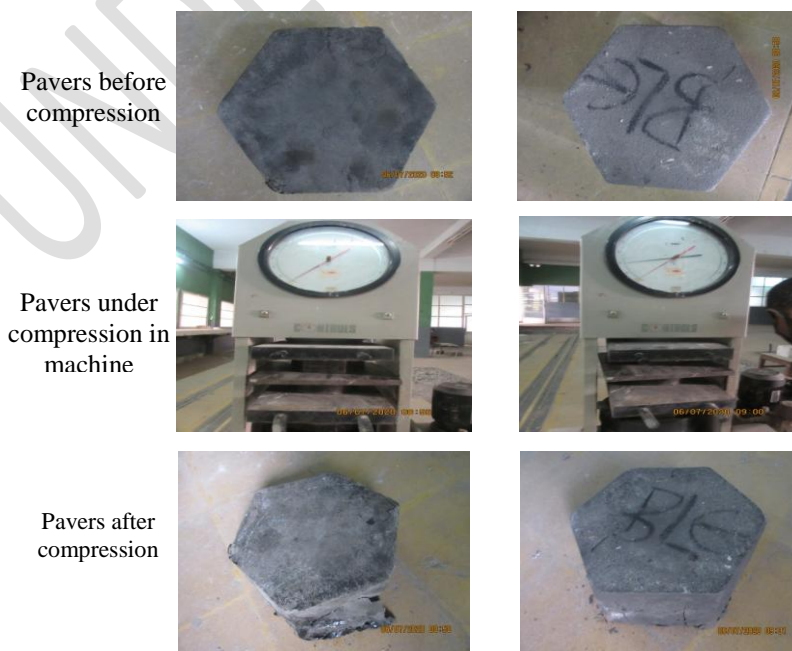
Figure 3. Reaction of pavers subjected to resistance testing
