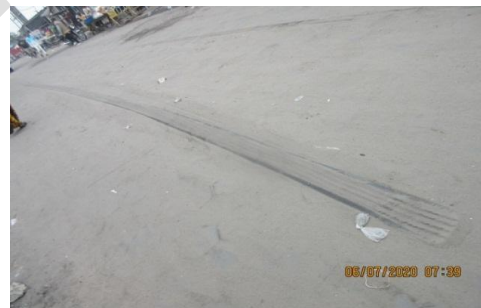
Close view of the engine brake traces
