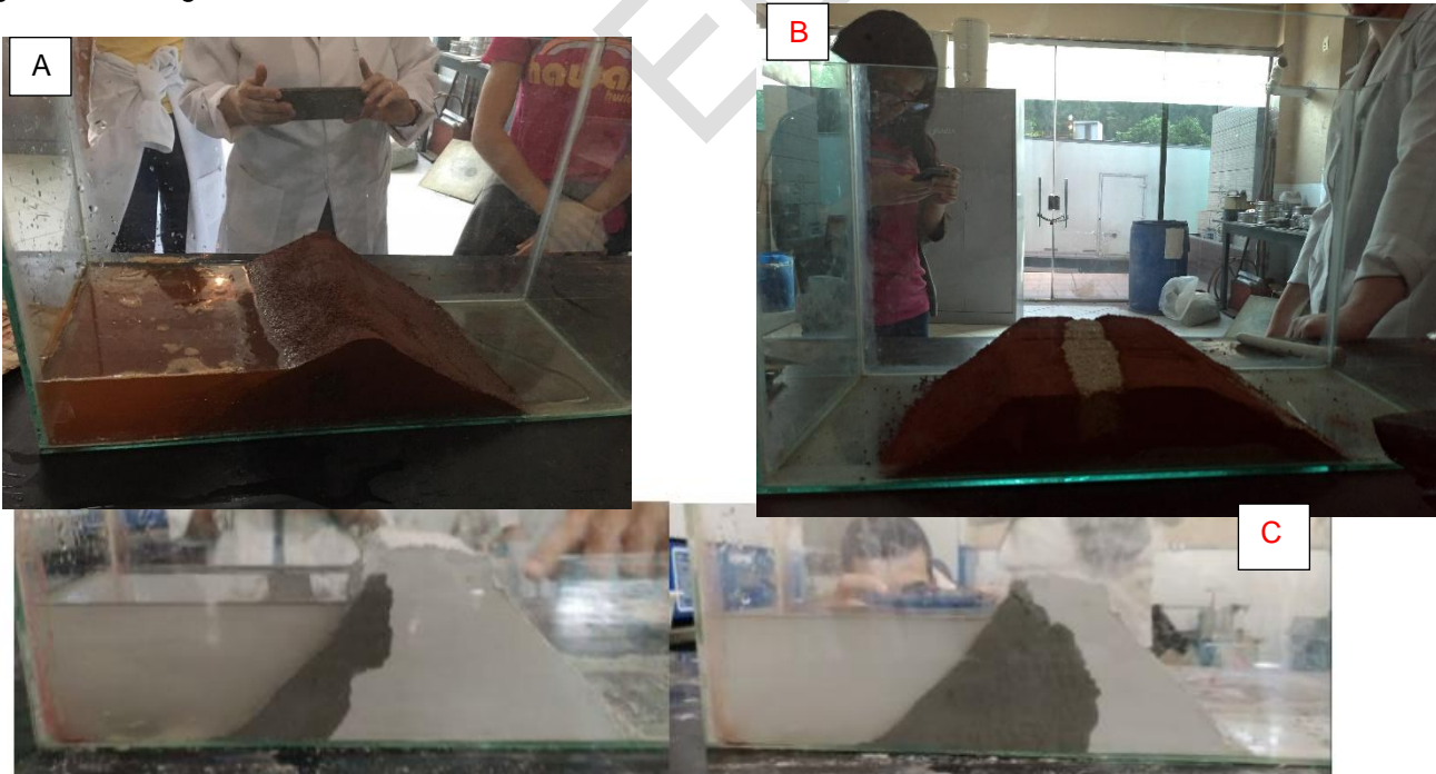
Figure 2- Construction of earth dam by students- A- homogeneous earth dam, B- earth dam with vertical drainage, C- tailing dam
