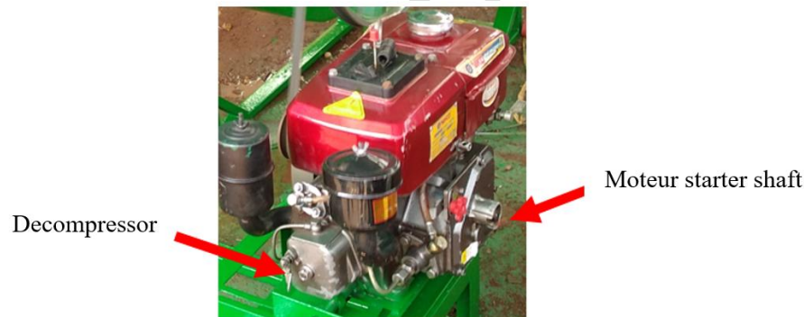
Fig. 6. Winnower motorization system
