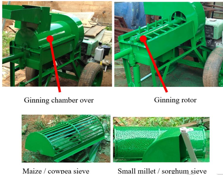
Fig. 2. Sheller adjusting devices
