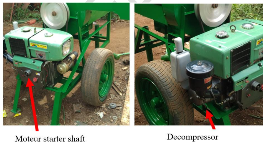
Fig. 3. Sheller motorization system
