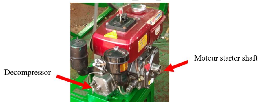
Fig. 6. Winnower motorization system
