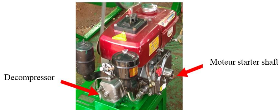
Fig. 6. Winnower motorization system
