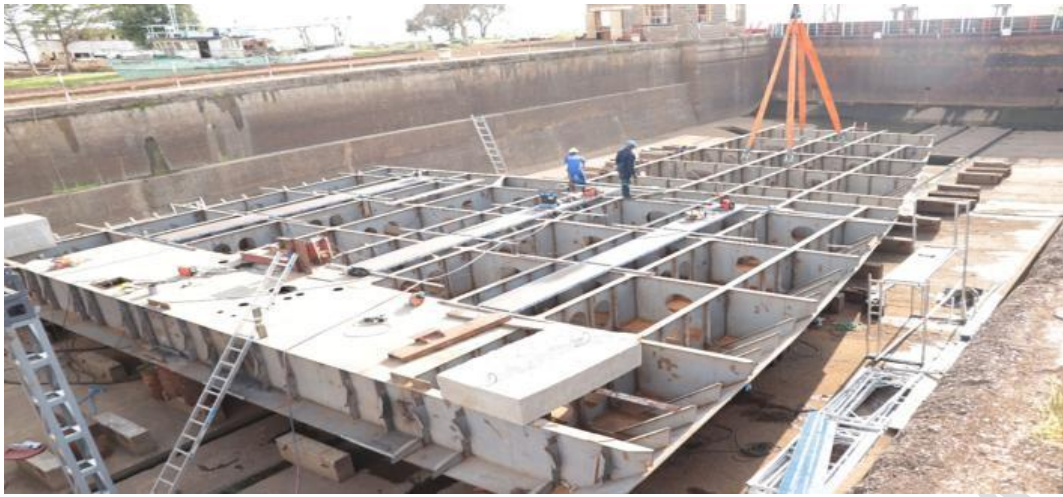
Fig-16 Installation of upper deck section
