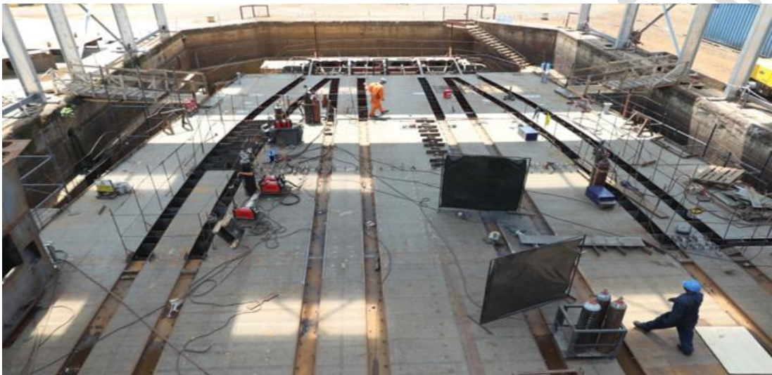
Fig-16 Installation of upper deck section
