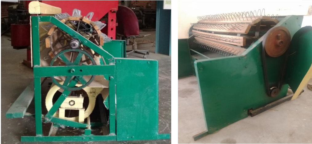
Fig (5):- Right Side and left Side View of pedal cum power Operated hybrid Thresher (case- 2)
