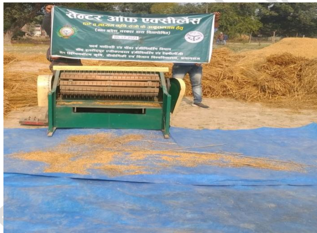
Fig6: Developed Pedal cum Power Operated Hybrid Thresher
