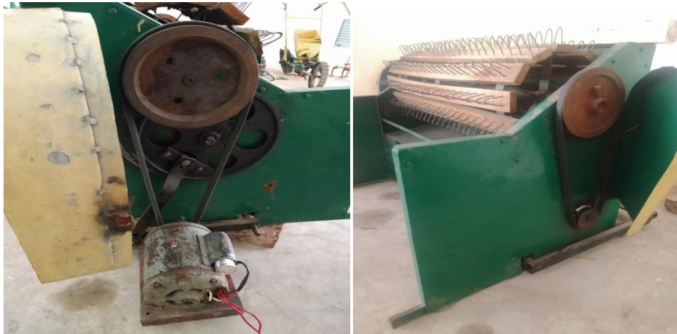
Fig (3):- Right Side and left Side View of pedal cum power Operated hybrid Thresher
