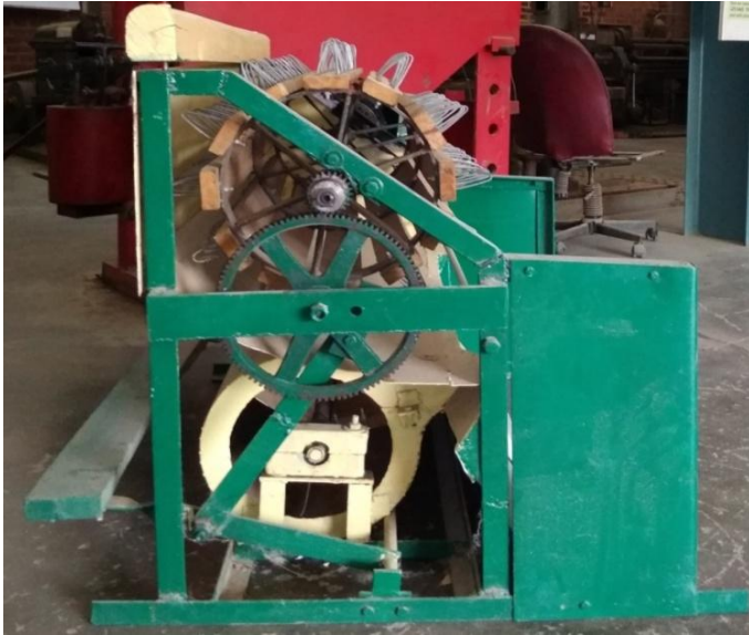
Fig (5):- Right Side and left Side View of pedal cum power Operated hybrid Thresher (case- 2)
