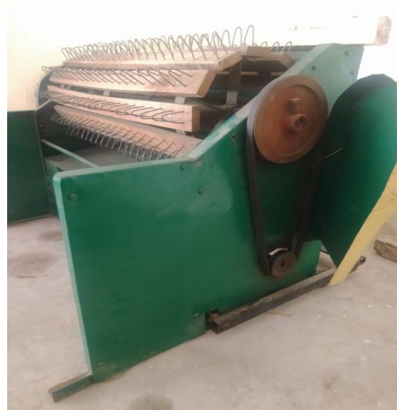
Fig (5):- Right Side and left Side View of pedal cum power Operated hybrid Thresher (case- 2)
