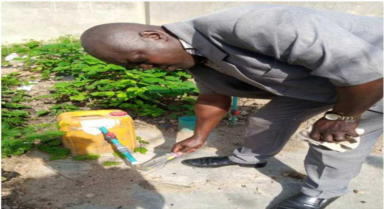
Fig 9: Researcher testing the flame coming out of the methane chamber with lighter
