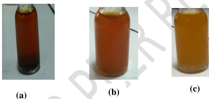
Picture 1. Viscera oil extracted at viscera/water ratio of 100:100, at cooking time 25min (a), cooking time 15min (b) and cooking time 10min (c).
