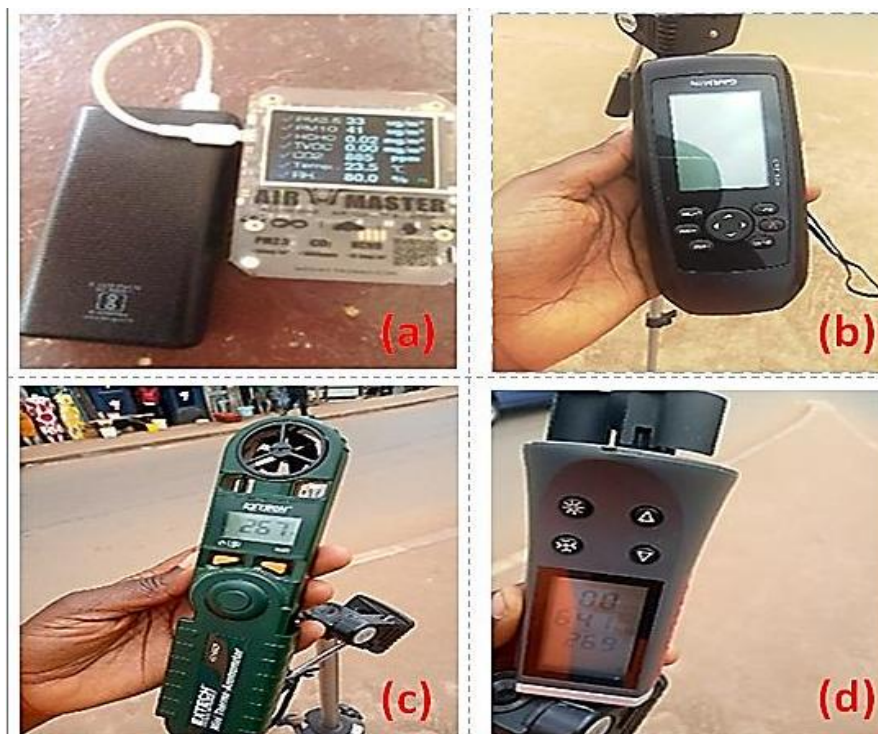
Fig. 2. The different devices needed for this study (a) Air analyser and charger, (b) Garmin type GPS, (c) Exttech, (d) Anemometer.
