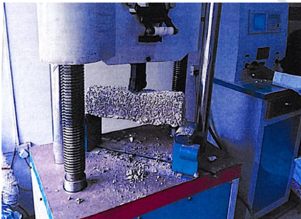
Fig 3. Prism specimen undergoing flexural test
