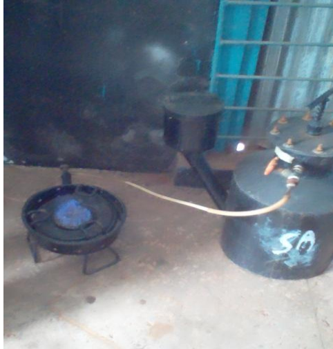
Fig 3: Flammability check using a gas burner
