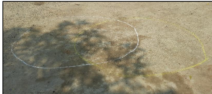
Fig. 2. Measurement of a spray overlap
