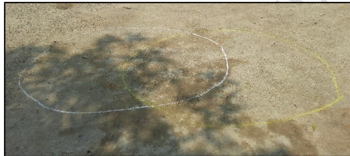
Fig. 2. Measurement of a spray overlap
