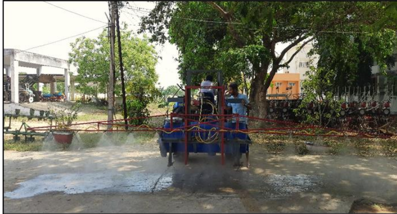
Fig. 1. Measurement of swath width of the tractor-operated boom sprayer
