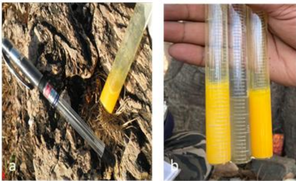
a. In field test of stromatolitic Limestone with Shapiro. S kit. The yellow colour suggests presence of P_2O_5 . b. Different intensity of yellow indicates varying percentages of P_2O_5 in the rock.
