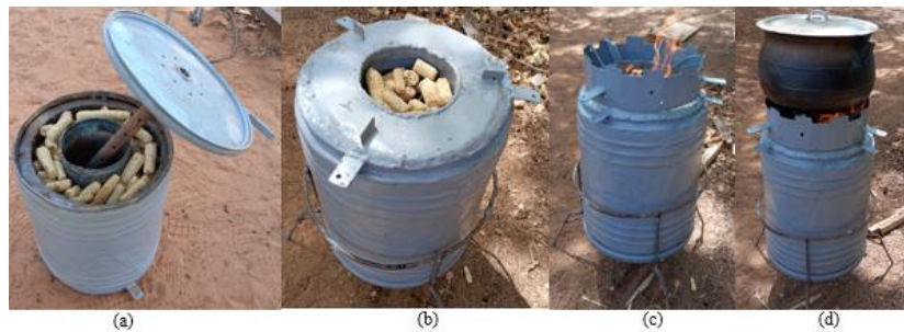
Figure 4: Principle of use of the multifunctional family oven
