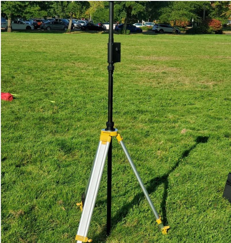
Figure 3. DJI D-RTK 2 high precision GNSS mobile station.
