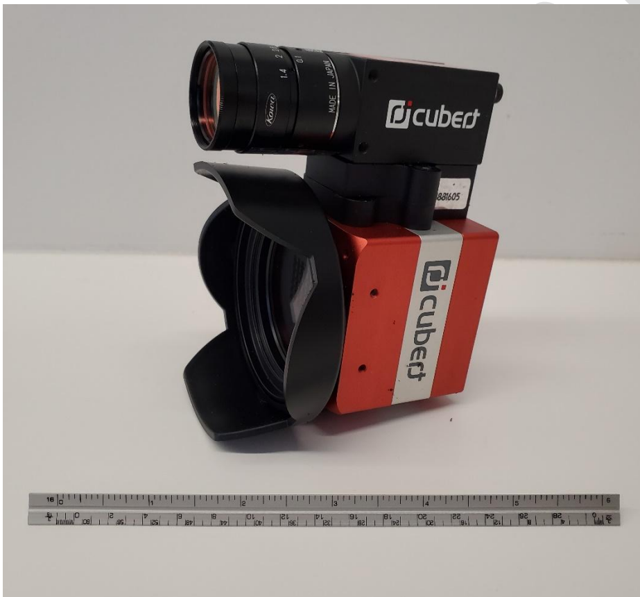
Figure 1. Cubert ULTRIS X20 Plus hyperspectral sensor. Ruler is approximately 16.5 cm in total length.
