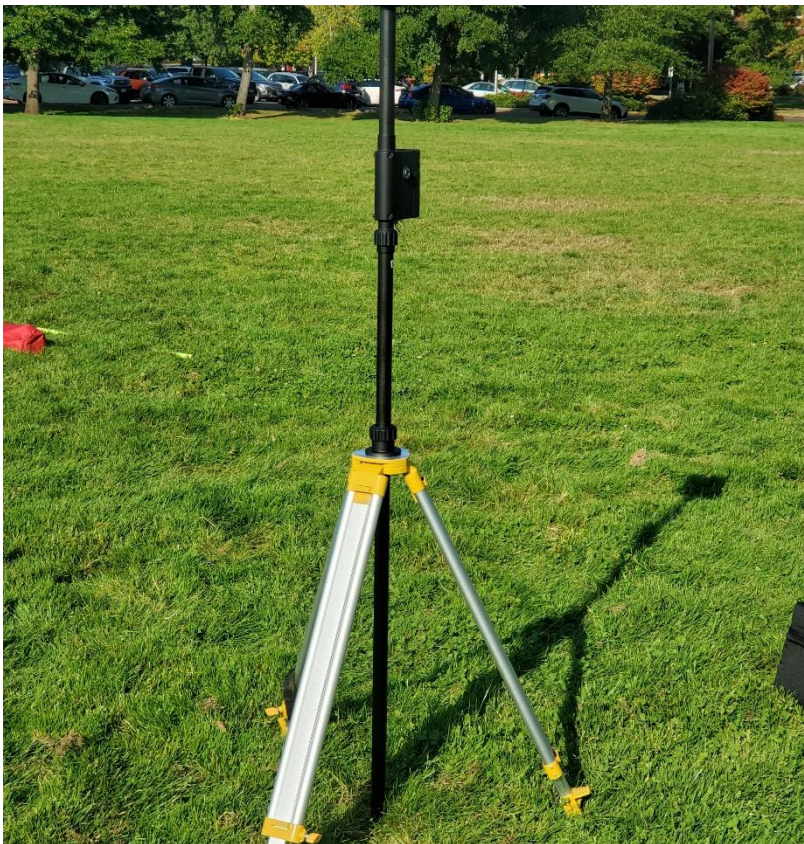
Figure 3. DJI D-RTK 2 high precision GNSS mobile station.
