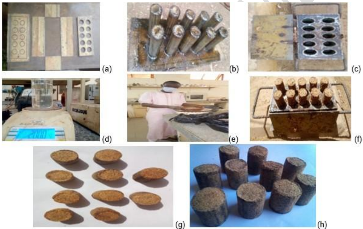
Figure 1: A cross-section of moulder and briquette making processes: (a) Plate cutting process (b) Base plate (c) Constructed Moulder (d) Water mass measurement (e) Sawdust sieving process (f) Briquette production (g) Sun-drying process (h) Produced briquettes
