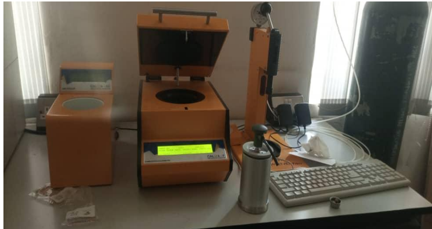
Figure 3: CAL3K-F Oxygen Bomb Calorimeter set up.
