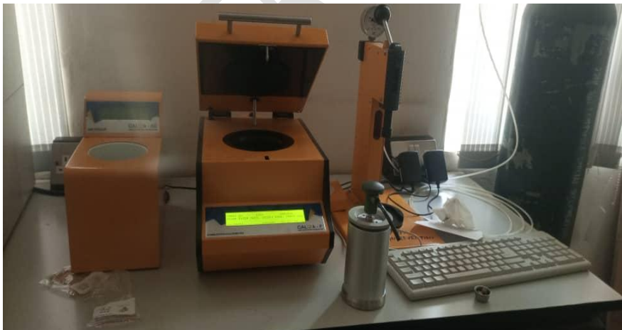
Plate 2: CAL3K-F Oxygen Bomb Calorimeter set up.
