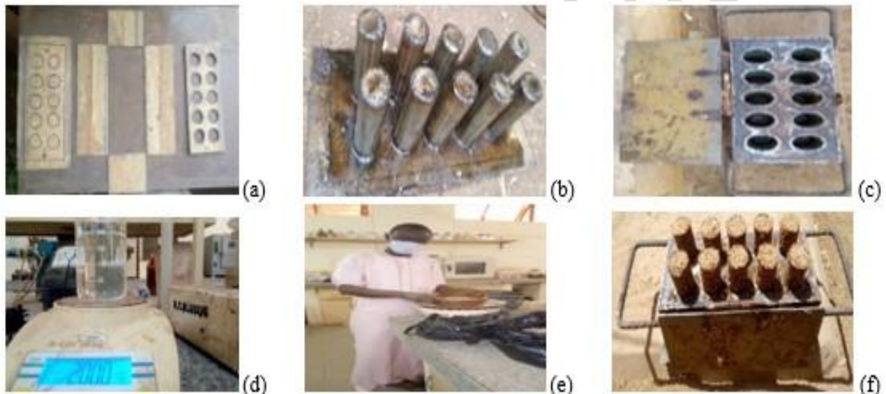
Plate 1: A cross-section of moulder and briquette making processes: (a) Plate cutting process (b) Base plate (c) Constructed Moulder (d) Water mass measurement (e) Sawdust sieving process (f) Briquette production
