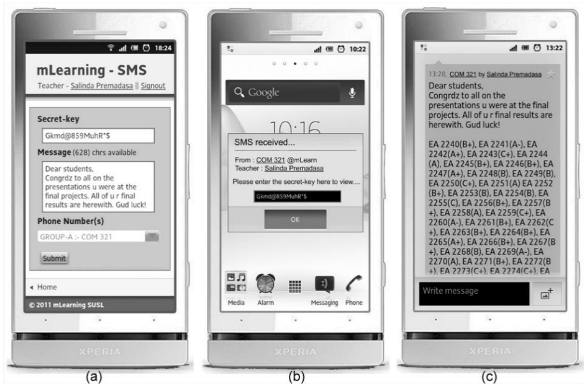
Figure 3. Front-end interfaces of the proposed system of the mobile phone with, (a) teacher inserts extensive text message with a secret key, (b) student receives the message and inserts secret-key, (c) student views the original message.
