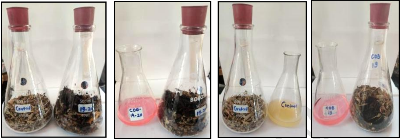
Plate 1. Results of CO 2 evolution test
