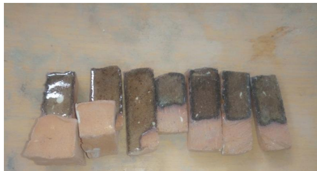
Figure 7: Test Result after Adjusting Runny
