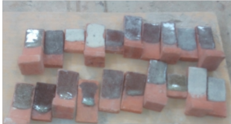
Plate 2: Test Blend Result of Files glaze number 11-26
