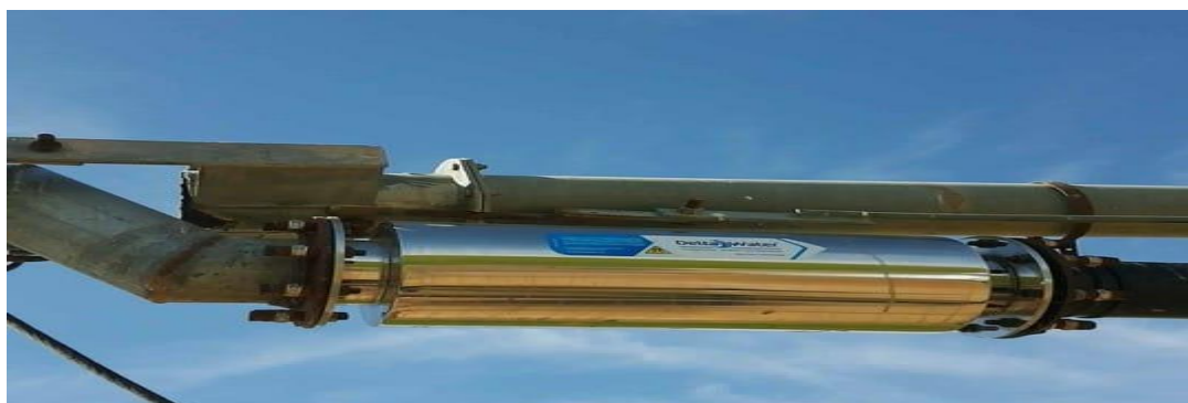
Fig (1). Magnetic system during irrigation water salinity study.
