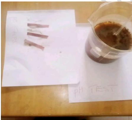
Fig 2: Soil Sample showing different pH test with litmus paper.
