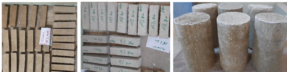
Figure 3: Prismatic and cylindrical specimens manufactured for testing
