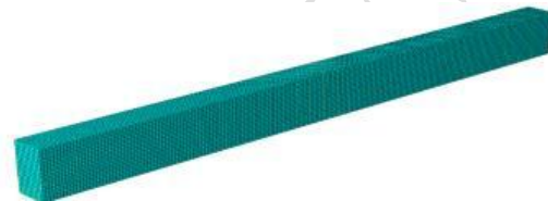
Fig. (6). Mesh Configuration of Finite Element Model
