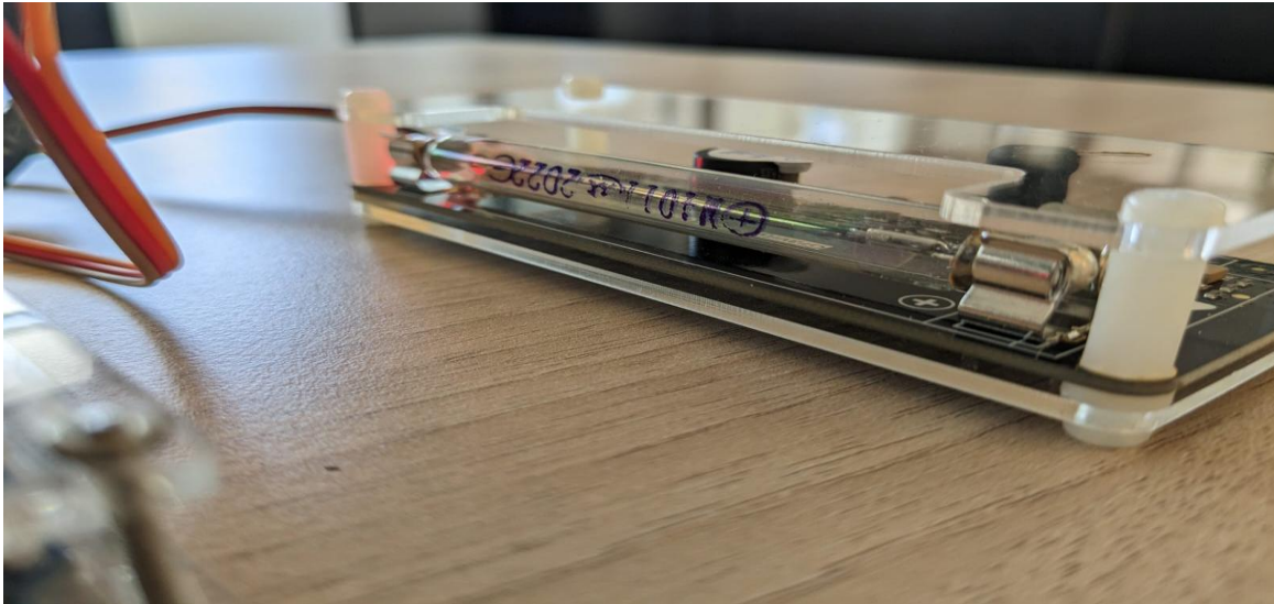
Figure 3: A Geiger tube with assembled Geiger counter circuit
