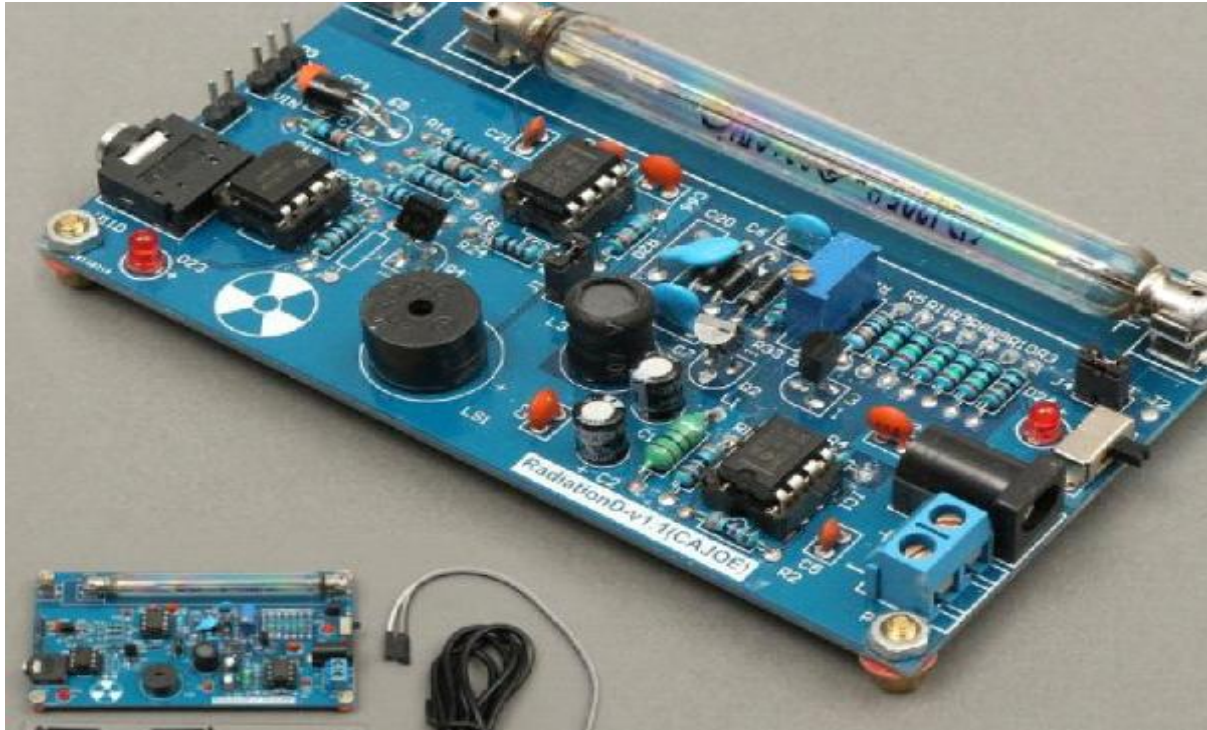
Figure 2: Radiation Detector (CRs) Circuit
