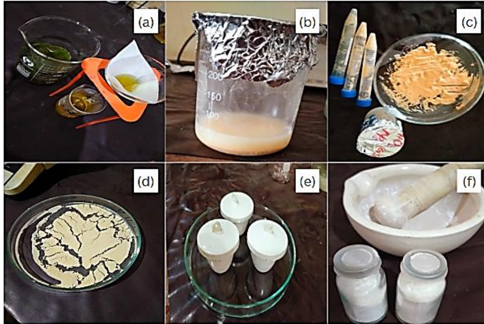
Fig 1. Green Synthesis of TiO 2 nanoparticles (a) Ziziphus mauritiana leaf extract, (b) layers formation, (c) centrifugation, (d) dried powder, (e) calcination, (f) TiO 2 nanoparticles
