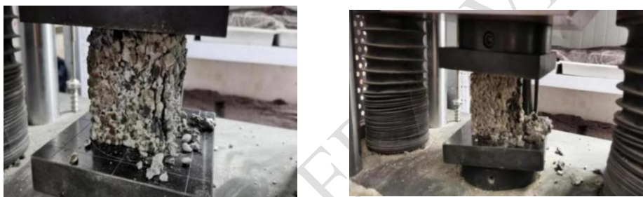
(a) Natural aggregate pervious concrete specimens (b) Recycled aggregate pervious concrete specimens
