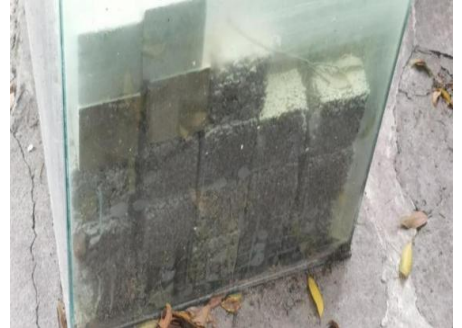
Fig 2. Recycled aggregate pervious concrete mixed with fly ash
