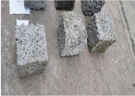
Fig 1. Pervious concrete with natural aggregate mixed with fly ash
