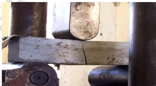
Figure 1. Bending specimen after loading
