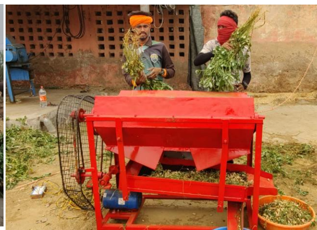
Fig. 10 Final testing for groundnut pod stripper
