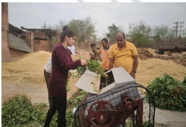
Fig. 9 Preliminary test of groundnut pod stripper
