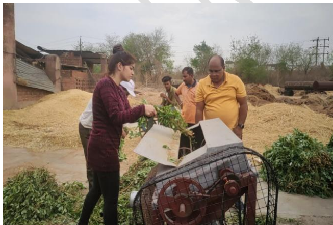
Fig. 9 Preliminary test of groundnut pod stripper
